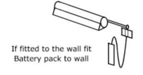
If light is fitted to frame the battery pack can still be fitted to the wall
