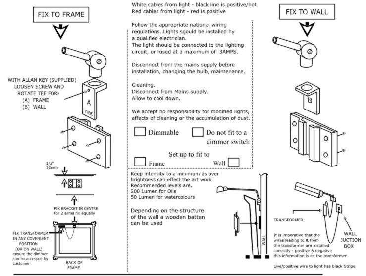
The Classic light is made to be light in weight - it is vital that the arms and swivels are loose when fitting and adjusting - if stressed the arm can fracture
